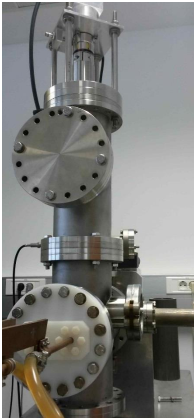
BBT with inductive heating system
