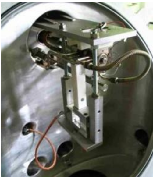
Image of the Ultra High Vacuum Tribometer: Internal View showing the Tribo-System with ball holder and disc
