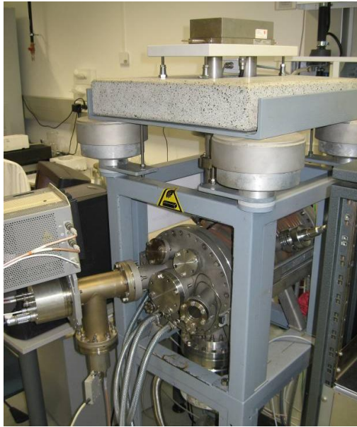
Sublimation test facility vacuum-balance (on top), vacuum chamber, quadrupole (left), turbo-pump (bottom)
