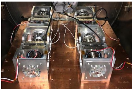
“BBT2”: 4 setups using frameless motor to test a pair of preloaded bearings, for long term and down to swivelling motions.
