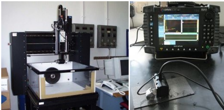
Figure 1: 4-axis ultrasonic scanner from Panametrics (left) and portable Ultrasonic phased array system Omniscan MX from Olympus (right)
