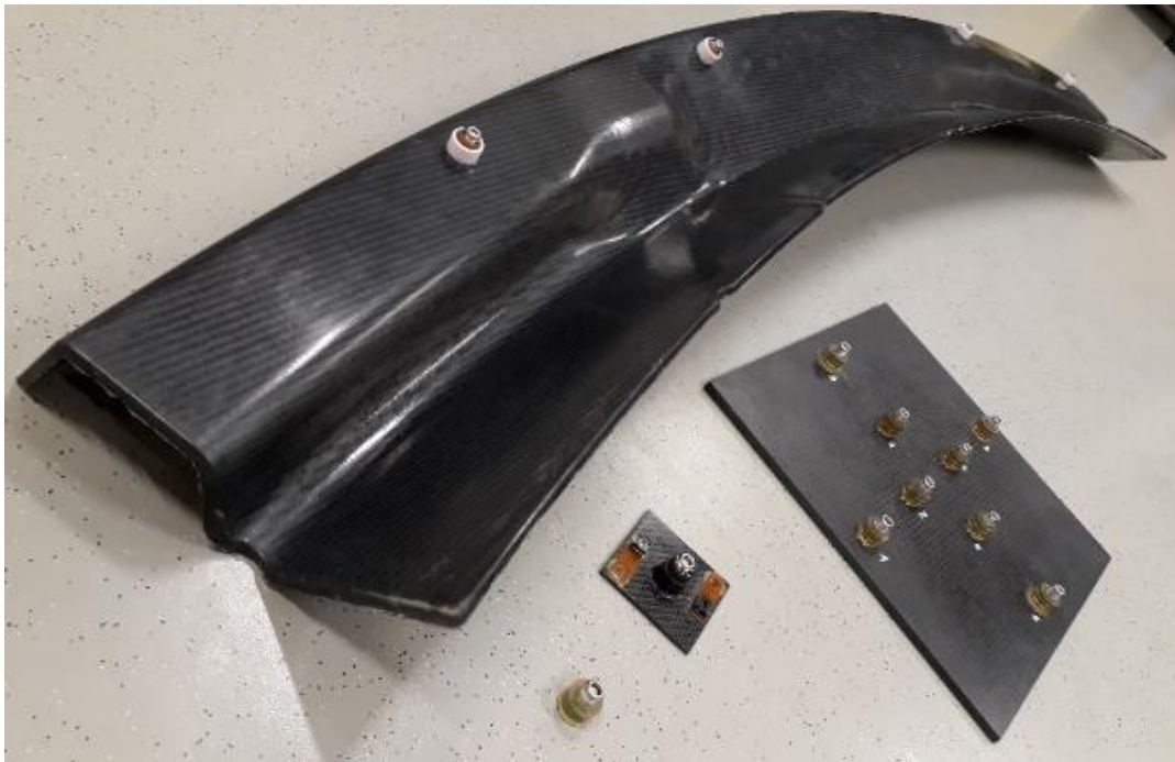
Figure 2: AAC Piezo Sensor and parts with integrated AAC Sensors for production and usage monitoring
