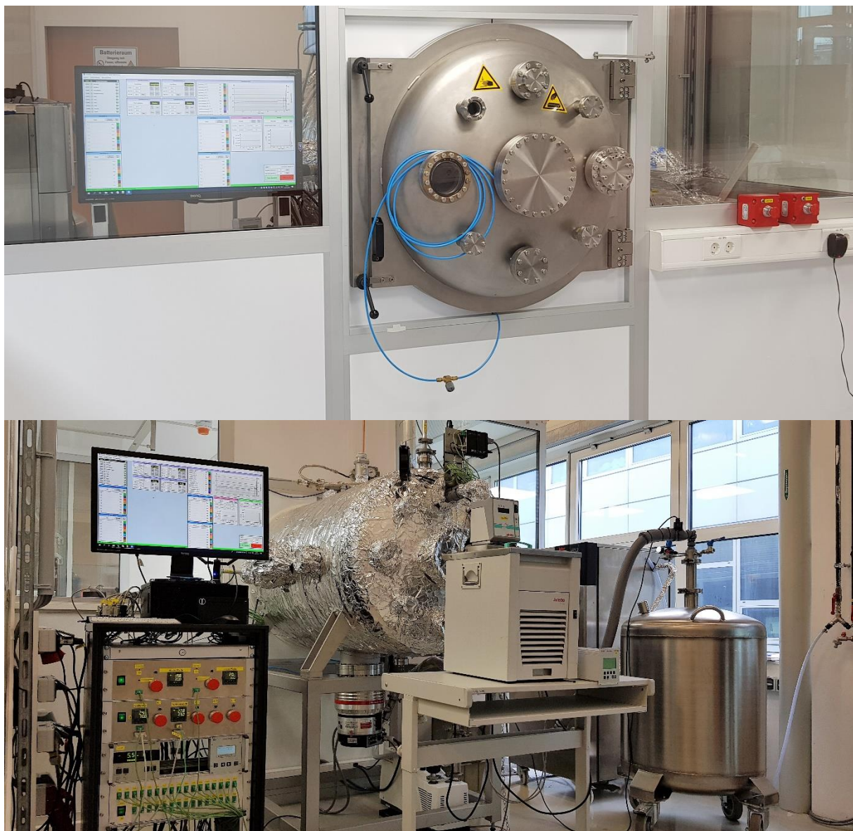
Figure 1: Overview of TVC Thermal Vacuum Chamber: up: view from clean room, down: view from laboratory.
