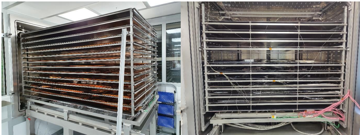
Figure 3: Bake-Out Jig, e.g., for MLI Bakeout: left – outside chamber during loading; right – inside XVC before closing main door
