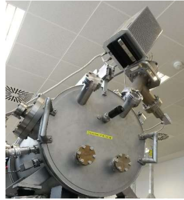
Figure 2: Vacuum tribometer with high temperature spindle and equipped with mass spectrometer
