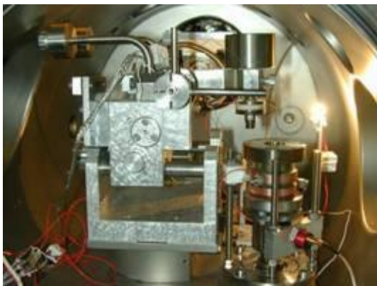
Figure 2: Vacuum tribometer with high temperature spindle and equipped with mass spectrometer
