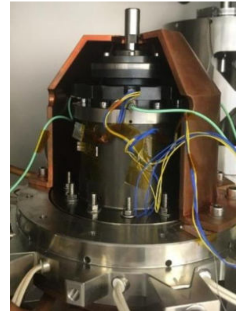
AAC test device "HADES" with test box for Harmonic Drive ® Gears
