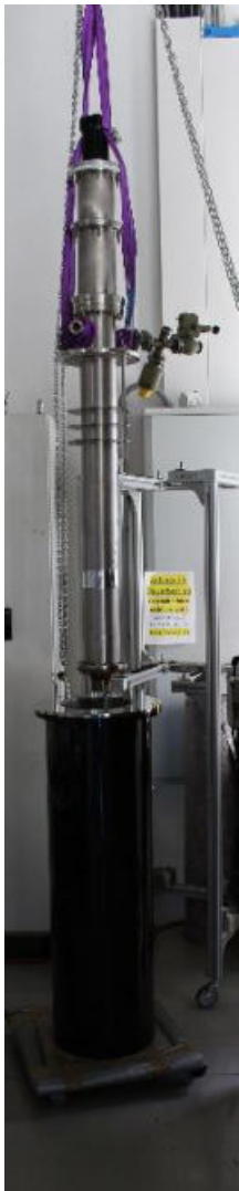
Vacuum Tribometer for cryogenic temperature testing
