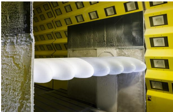
Icing wind tunnel test of wing mockups with anti-icing and reference coatings side by side.
