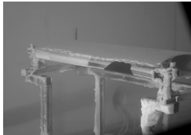
Electro expulsive de-icing system and passive anti-icing coating in icing test.
