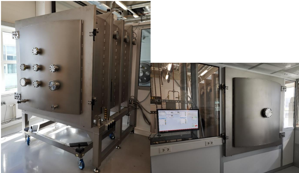
Figure 1: Overview of XVC Thermal Vacuum Chamber: right: view from clean room, left: view from test center.
