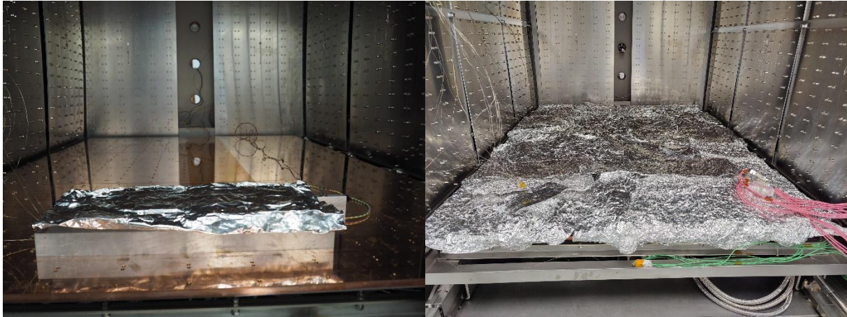
Figure 2: View inside XVC Thermal Vacuum Chamber: left – small component installed; right – parts under Al foil insulation
