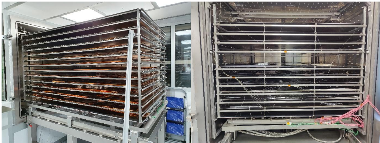
Figure 3: Bake-Out Jig, e.g., for MLI Bakeout: left – outside chamber during loading; right – inside XVC before closing main door
